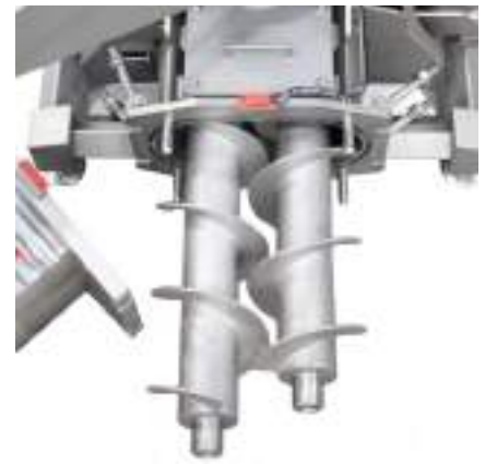
Close up view of twin screws, top view.
