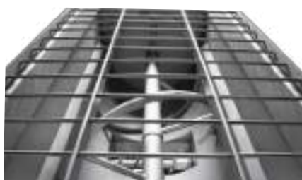
2500 L silo/buffer hopper with stirring/feeding device. The stirring device feeds product to the centre for discharge into SuperPump SP 200.
