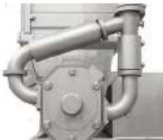
SuperPump SP 290 showing double pump discharge.
