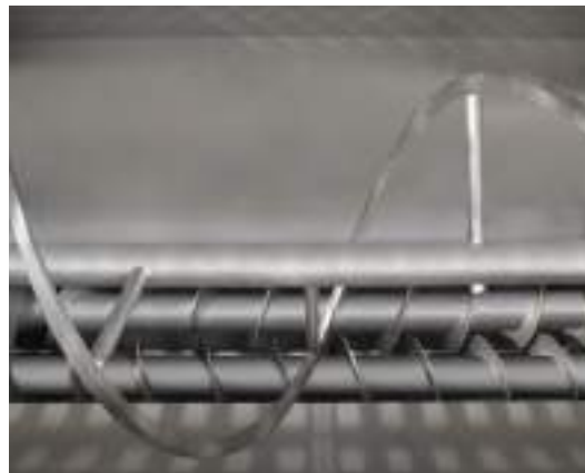
Top view and inside look of the TSF. Both the twin screws and the feeding wing are shown.
