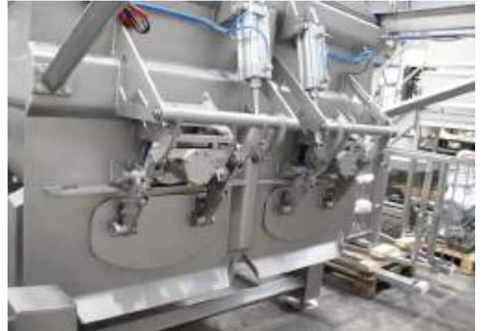
Details of scansteel foodtech® Heavy Duty Outrigger Shaft Seal System
