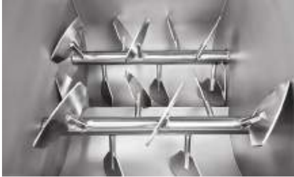
Optional mirror polished paddle mixing wings. Twin Shaft Mixer Intermeshing, TSMI Series.
