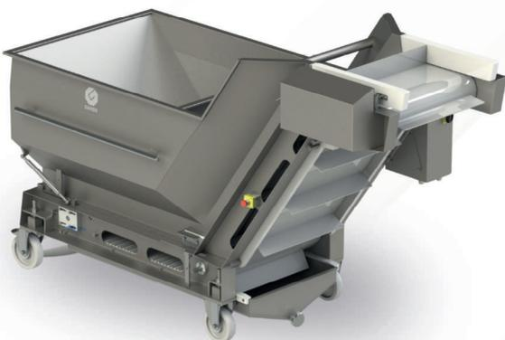
GAF (Garos Automatic Feeder) dispenses products an even layer, with capacity adjusted to suit the injector. The GAF has a volume of 800 l which allows for a full 800 l bin to be emptied into the trough. The feeder is equipped with a collection tray for product drip-off, which can optionally be transported by pump to any other location. For more information, please check our GAF brochure.
